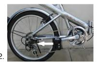
2. Rotate the crank so that the folded pedal is pointing toward the rear wheel. (For Latte, you have to lift up the rear wheel off the ground and rotate the crank in the forward direction)
