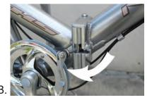
6. Open/Loosen the quick-release on the main body. Next, swing the quick-release lever toward the rear of the bike.
