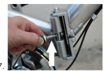
7. Pull up on the quick-release lever to release the safety pin, thus un-latching the folding mechanism safety pin.
