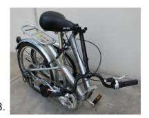
8. Fold the bike in half. If you have Mocha, be careful that the cables do not snag on the folding mechanism.
