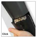
**INSTALLING THE BATTERY PACK.** We recommend standing on the left side of the bike.
