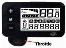
LCD dashboard content description Power output and battery level indicators section
