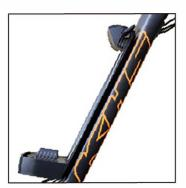
To remove the battery pack, we recommend that you stand on the left side to the frame. (Standing on the left side of the bike gives you more leverage)
